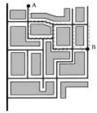
DEFORMED GRID LAYOUT Permeability high Choice of routes between A and B possible, and at least one of these routes is relatively direct
